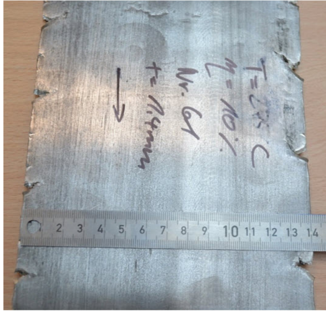
Fig. 13 Enlarged view of the edge cracks for sheet 61; typically, damage was limited with crack lengths of about 5 to 15 mm
