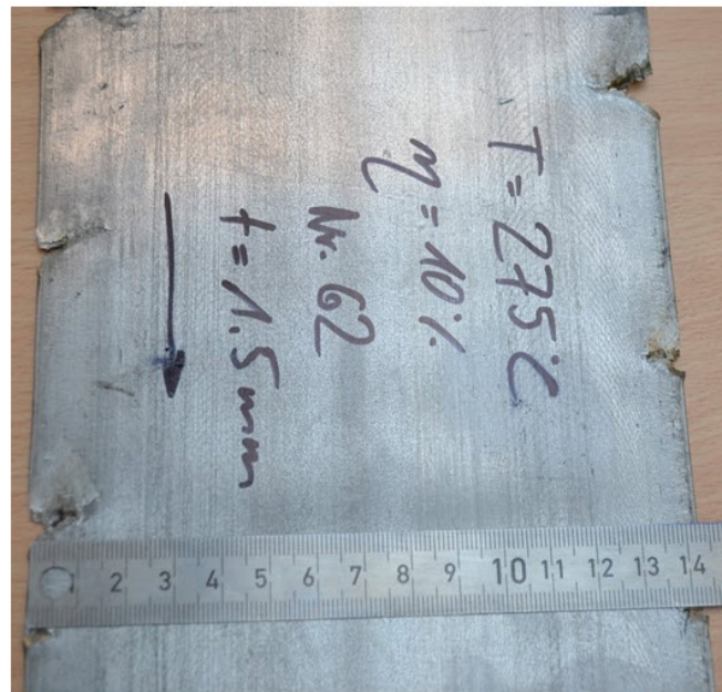
Fig. 14 Enlarged view of the edge cracks for sheet 62; typically, damage was limited with crack lengths of about 5 to 15 mm
