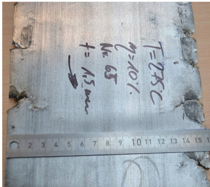
Fig. 16 Enlarged view of the edge cracks for sheet 65; typically, damage was limited with crack lengths of about 5 to 25 mm
