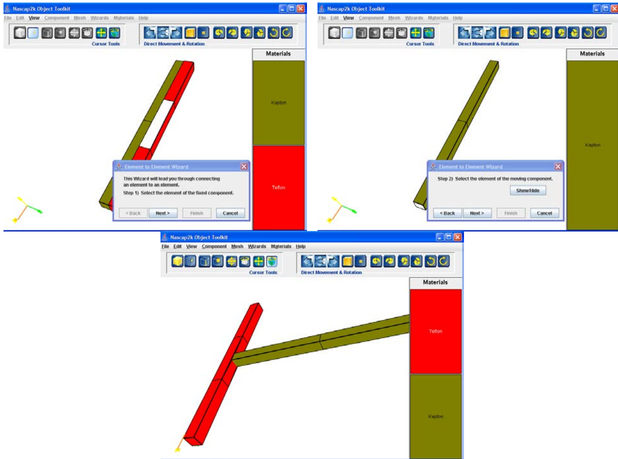
Figure 107. Joining Two Booms into a T Shape Using the “Element to Element Wizard.”
