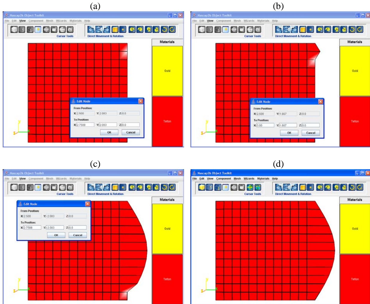
Figure 32. Changing the Edge of a Panel from a Straight Edge to a Cosine Curve by Repeated Use of “Edit Node” on the Mesh Menu.
