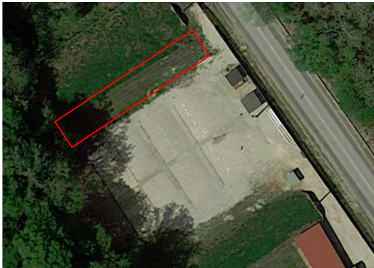
Figure 17. North Range Showing the Area that was Levelled to Accommodate Placement of the Flexible Reactive Barriers.
