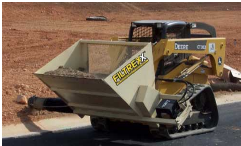
Figure 15. An Example of Commercial Equipment Used for Filter Sock Assembly
