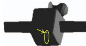
Fig. 19. Beginning of panoramic map. LRF strike points are shown inside ellipse, with first strike points indicated by arrow.
