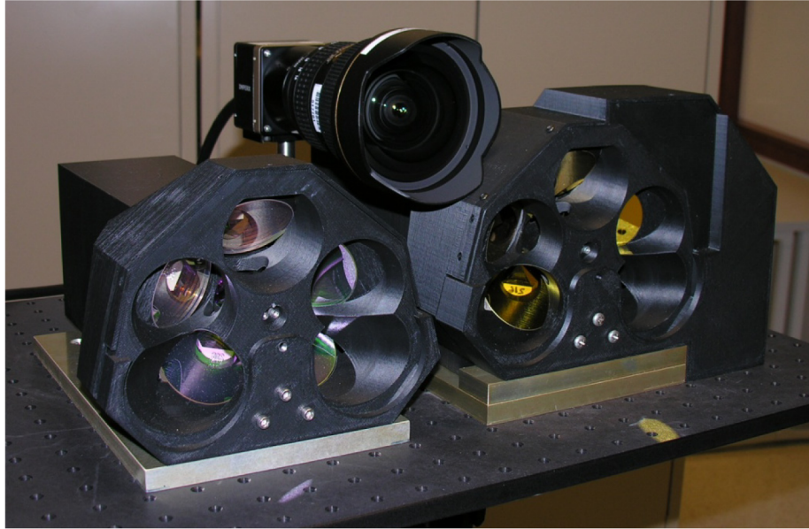
Fig. 7. SWIR five-channel prototypes. Left: SWIR prototype 2 with a wedged dichroic fold mirror for spatial encoding. Center: a visible witness camera. Right: SWIR prototype 1 with a metalized fold mirror and filter wheel.
