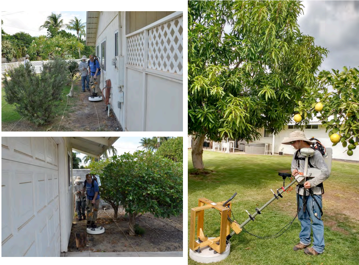
Figure 11: MPV dynamic and cued surveying at house 1: 69-1745 Puako Beach Drive.
