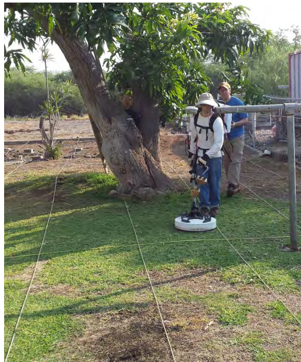
Figure 5: MPV operator surveying in dynamic mode following rope lanes. Operator follows straight lines.
