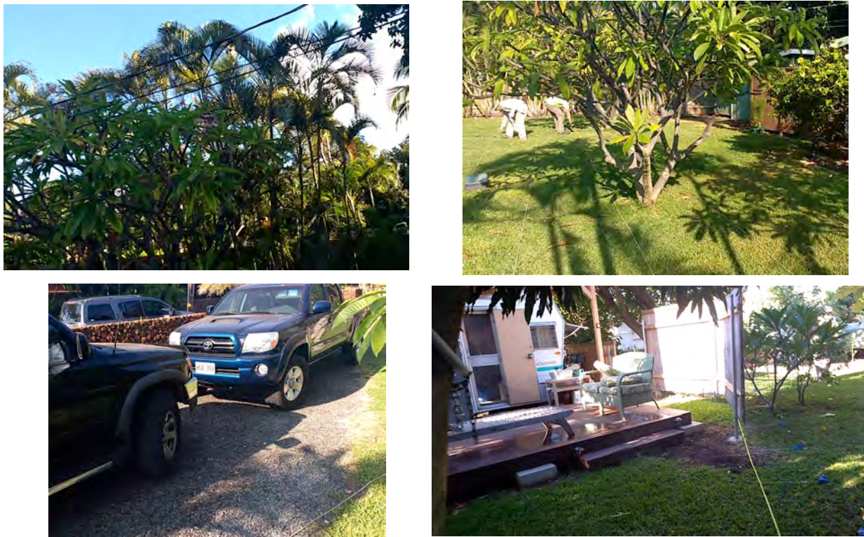
Figure 29: MPV dynamic and cued surveying environment at house 4: 69-1877 Puako Beach Drive. Significant tree canopy in the backyard meant RTK GPS surveying was not possible. Trees, vehicles, an office trailer and overhead power lines were some of the cultural targets present in the survey area.
