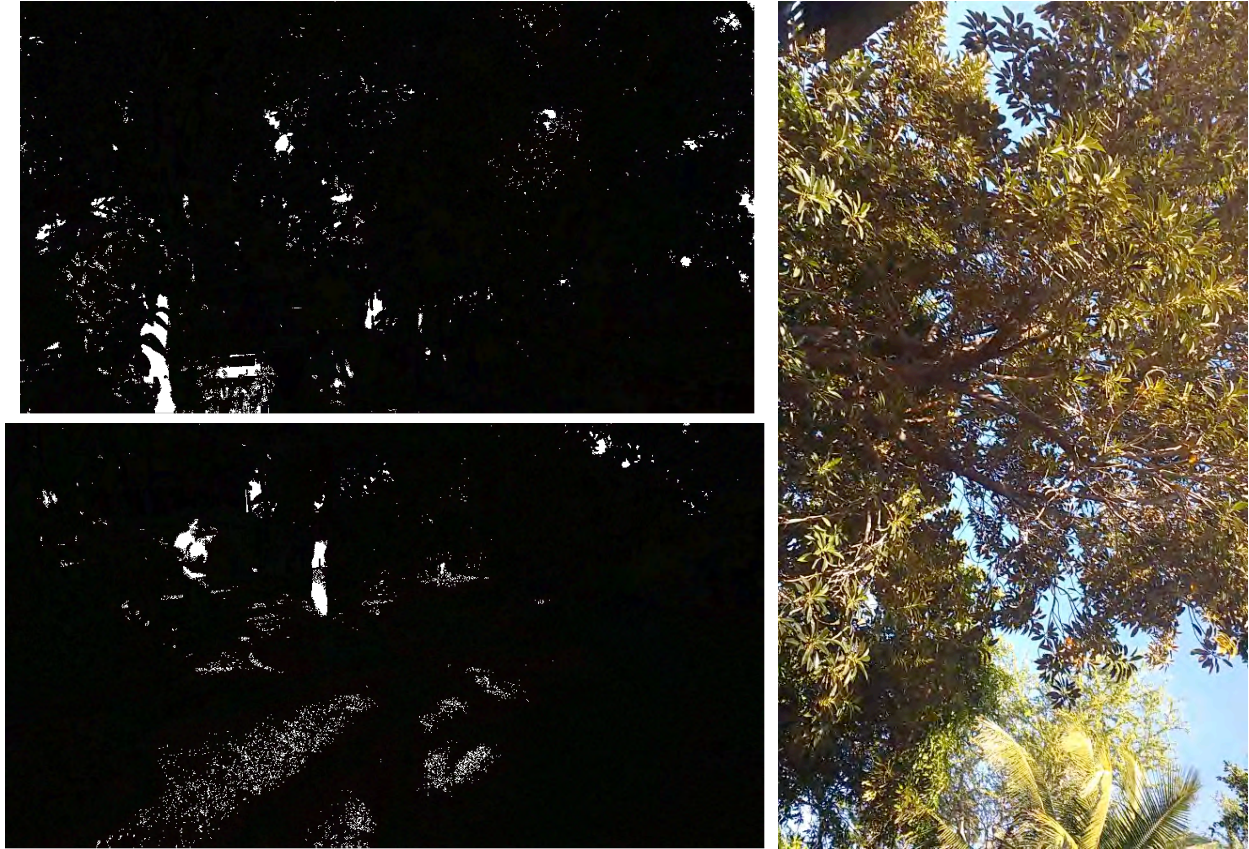
Figure 41: MPV dynamic and cued surveying environment at 69-1971 Puako Beach Drive. While the yard itself was relatively unobstructed, large trees around the perimeter created a canopy that covered virtually the entire property making RTK GPS surveying impossible.
