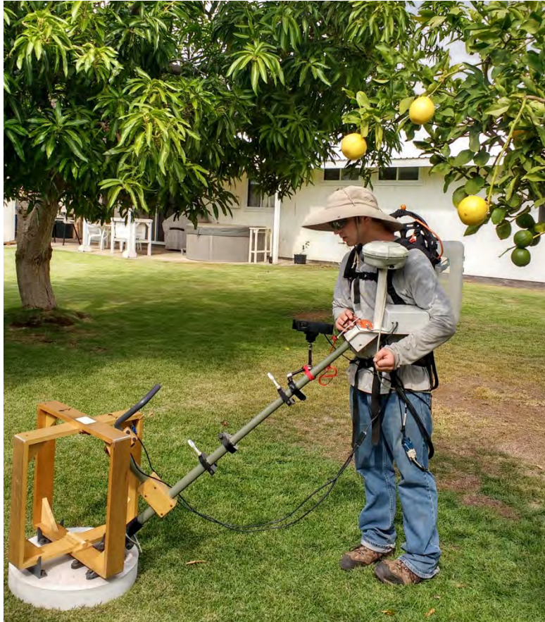
Figure 6: MPV3D cued interrogation. The first sounding takes place at the picked location. The data are inverted and a second measurement might be taken in the case of large predicted offset.
