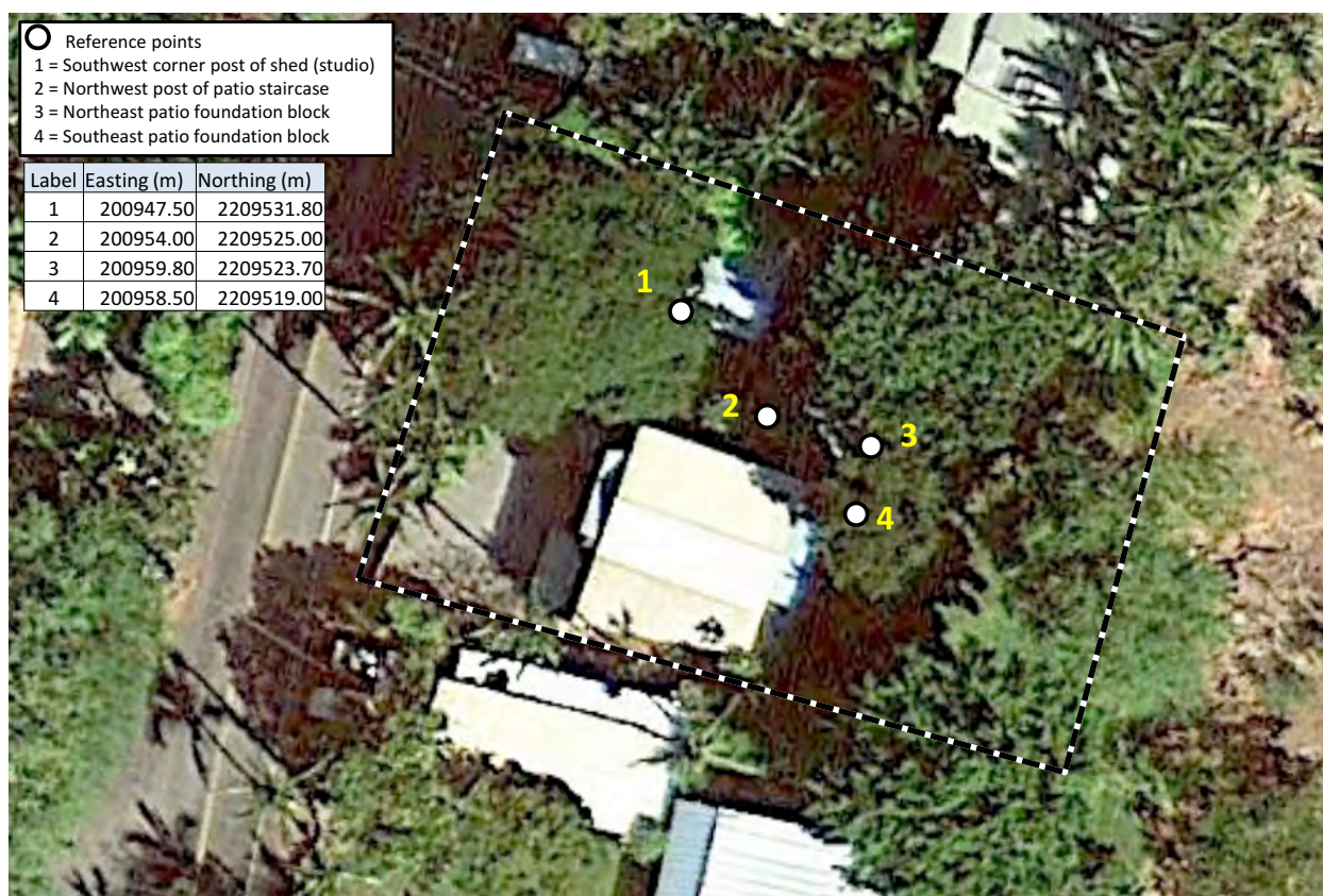
Figure 45: GPS co-ordinates for reference points used by field crews to position cued MPV3D measurements were identified in Google Earth in order to investigate performance against QC seeds at 69-1971 Puako Drive.
