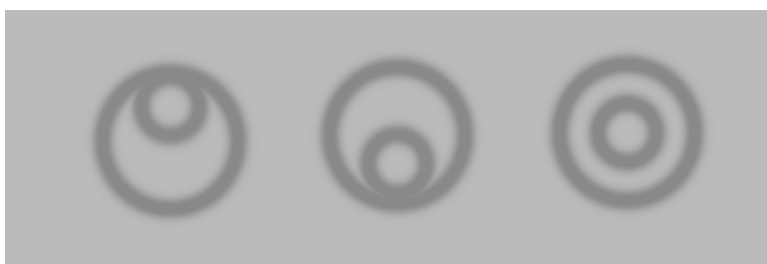
Figure 9. Examples of the positional tracking test in the up (right image), down (middle image), and correctly cancelled out center (left image) positions.
