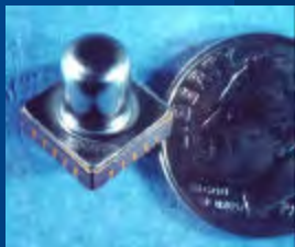
Low Energy EFI Detonator - Fully Qualified - Manufactured by Silicon Designs and Reynolds Systems
