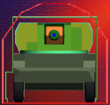
GENERIC FCS VEHICLE/RAMM IN C130 AND RAILWAY TUNNEL GAGE
