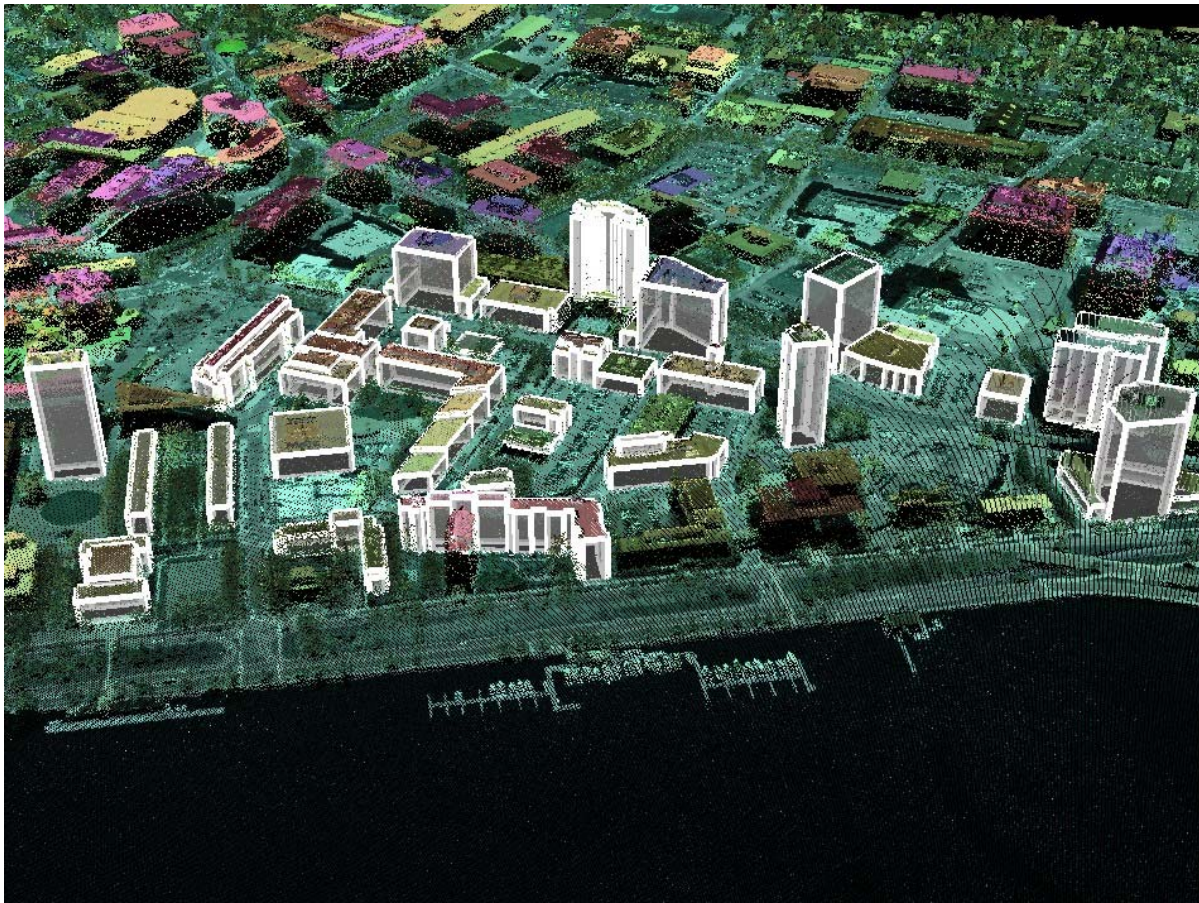
FIGURE 7. Building models are superposed against the lidar point cloud fused with the orthorectified aerial image.
