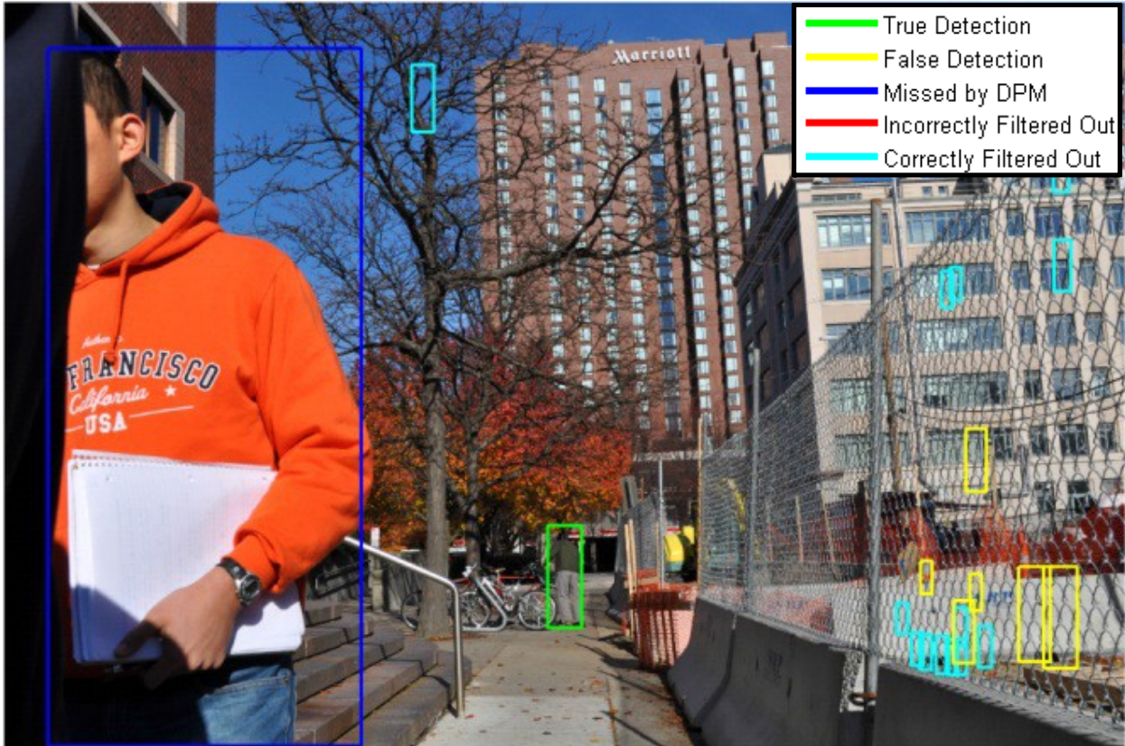
FIGURE 22. Detection results after applying the false-alarm filters are shown in the image space. About 20 detections were made. The one true detection is in the green box. The DPM algorithm missed the person on the left because he is partially obscured. The cyan boxes show the cases in which the false-alarm filters correctly eliminated those detections.
