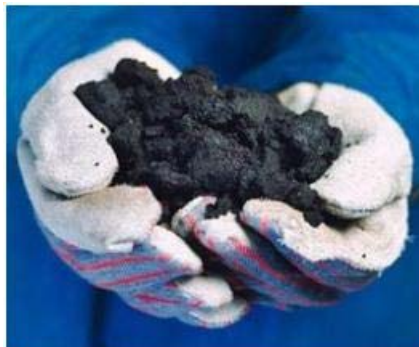
Figure 1. Bitumen, which can be diluted to become Dilbit crude oil.
