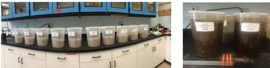
Figure C-2. “Weighed” crude oil aliquot directly into the 4.5 kg of dry sand, in the experimental container.
