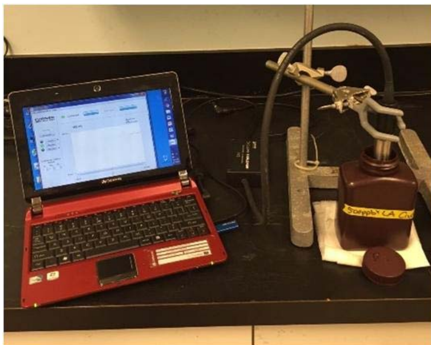
Figure B-2. Cyclops-7 laboratory calibration setup.
