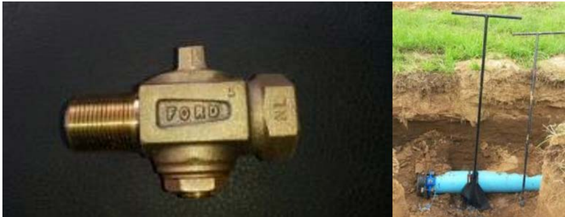
Figure 5-2. Simulated Leak Configuration Using Corporation Valves
