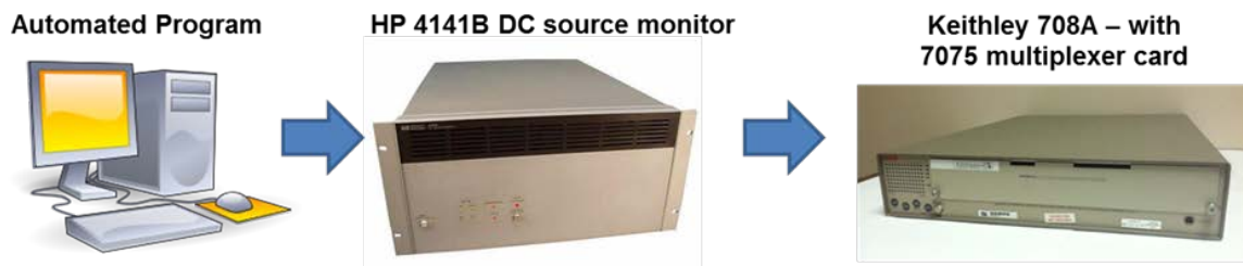
Figure 23. Test setup for in-situ measurement of ZnO TFTs modified for increased multiplexing capabilities.
