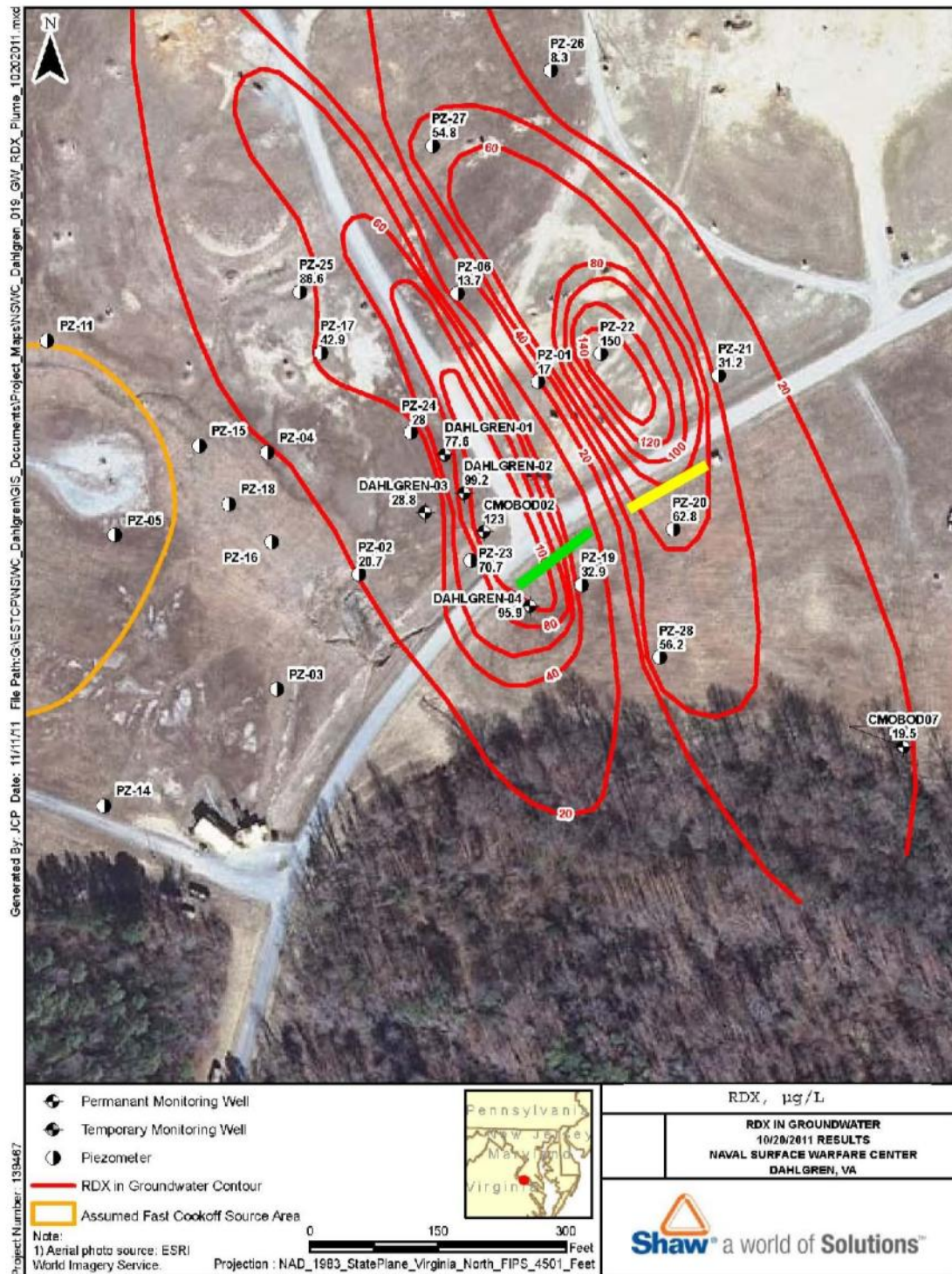
Figure 5.3. Plume Map for RDX in the Southeast Area of the Churchill Range.
