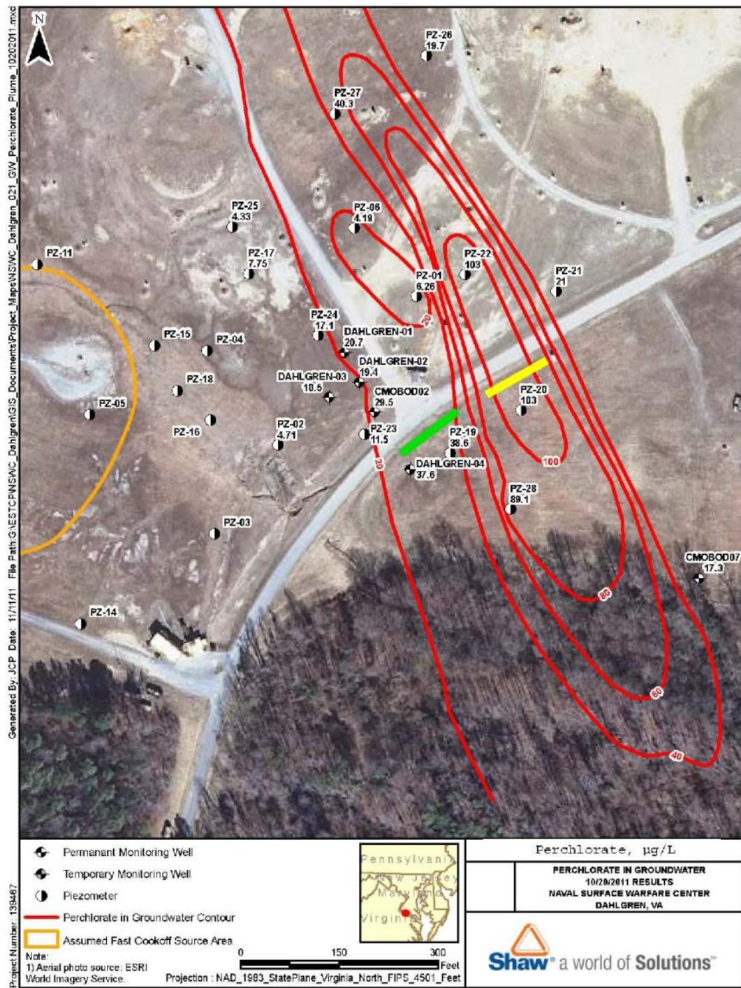
Figure 5.4. Plume Map for Perchlorate in the Southeast Area of the Churchill Range.
