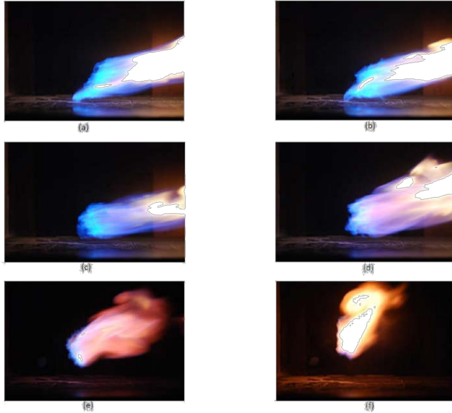
Figure 7: Flame luminosity images for partially premixed methane jet flame in crossflow, (a) Re = 1750 , (b) Re = 2000 , (c) Re = 3000 , (d) Re = 4000 , (e) Re = 6000 , (f) Re = 8300
