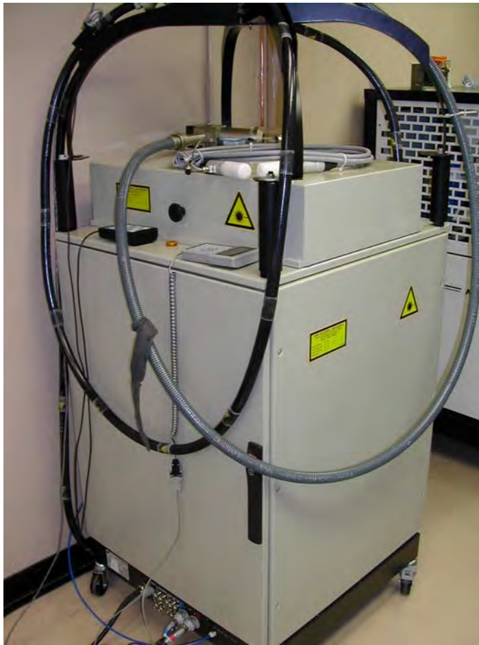
Figure 11: Quantel 40watt main system with the handheld unit resting on top. There is a remote to turn on the main system, then activate the handheld unit with the trigger. Note- no hanger or holster to secure the handheld unit.
