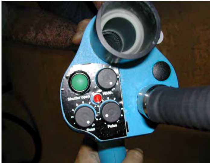
Figure 5: 120watt device- posterior side. Green button is pressed to initially start handheld unit. Top portal is for ventilation hose, bottom line is fiber-optic.
