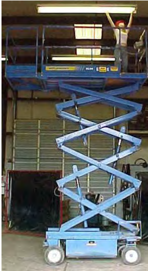
Figure 18: Scissor lift work platform
