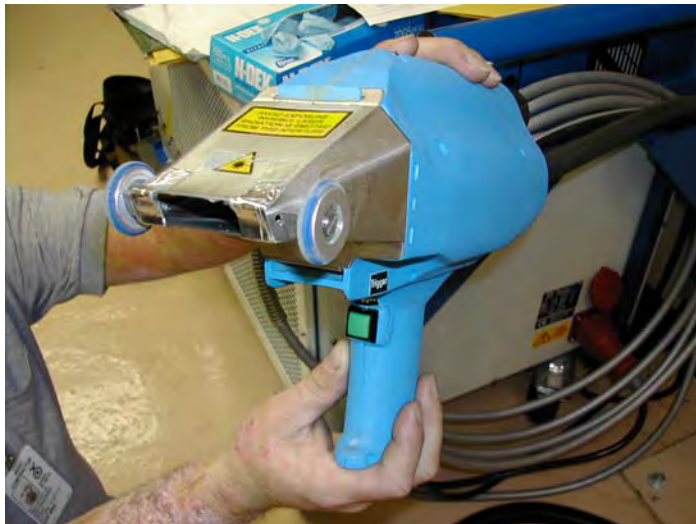
Figure 6: 120watt wheeled nozzle, unable to view small upper capture vent from this angle.
