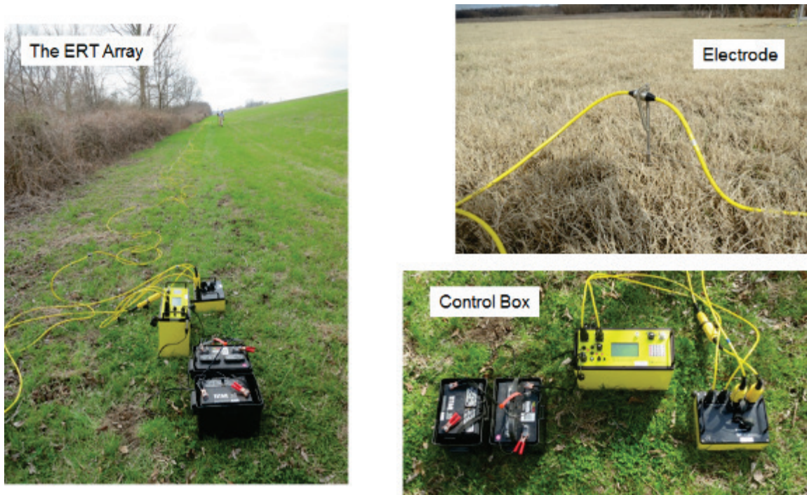
Figure 11. AGI SuperSting 8 ERT survey equipment.
