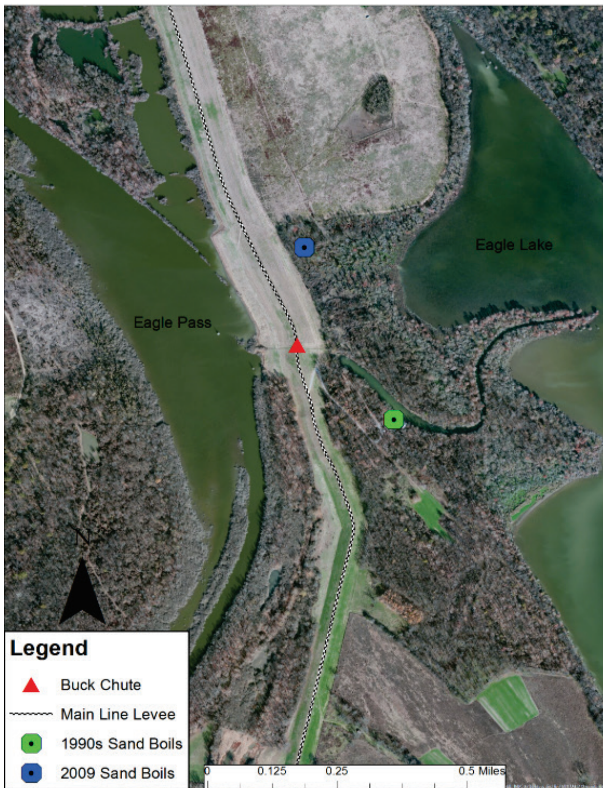
Figure 3. Aerial imagery of the immediate vicinity of the Buck Chute site with the locations of sand boils (Modified from World Imagery base map downloaded from ESRI ArcMap 10.1 library).
