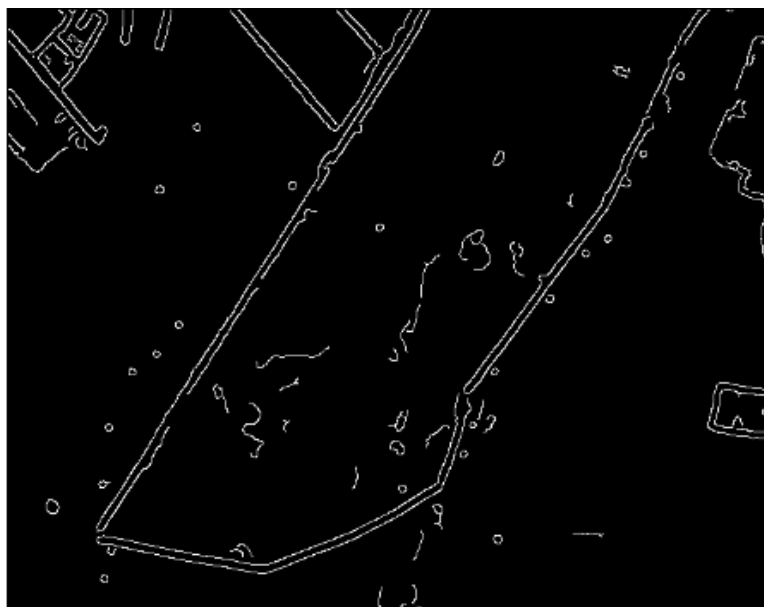
Figure 9. Result of the Canny edge detector. The algorithm did a good job picking out the edges in the smoothed gradient image.
