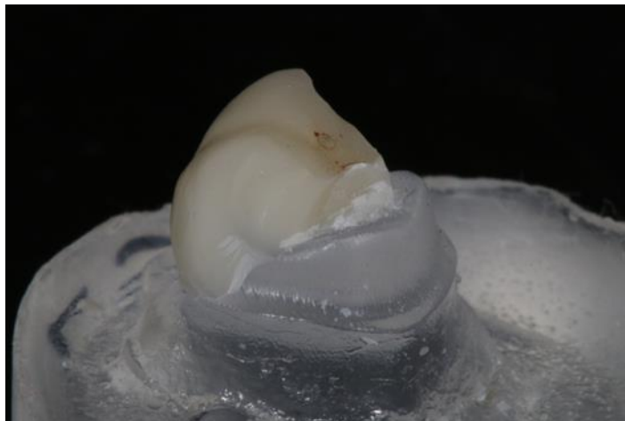
Figure 9. Fracture pattern showing catastrophic failure of the crown material with intact resin die.
