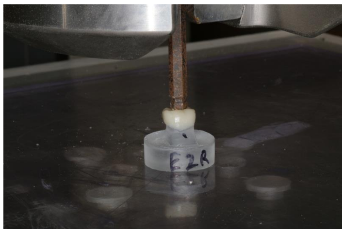
Figure 5. Positioning of sample for axial loading with The 858 Mini Bionix II.
