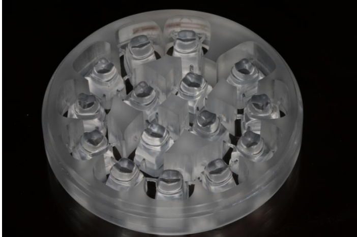
Figure 1. PMMA Resin Puck with 15 identical dies following milling process.
