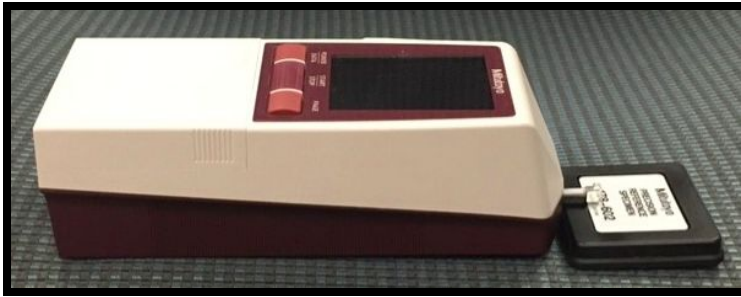
Figure 5: Surface profilometer surface roughness tester
