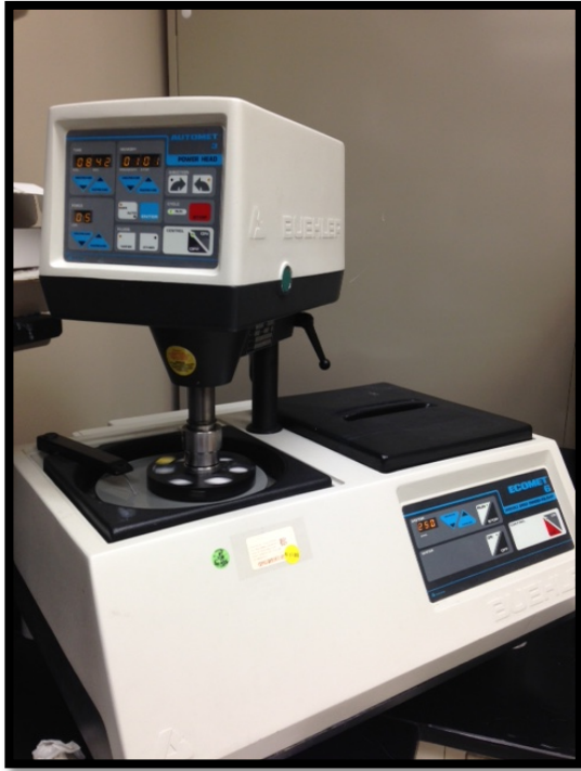
Figure 3-5 Six ring samples being polished on Buehler Ecomet 3.
