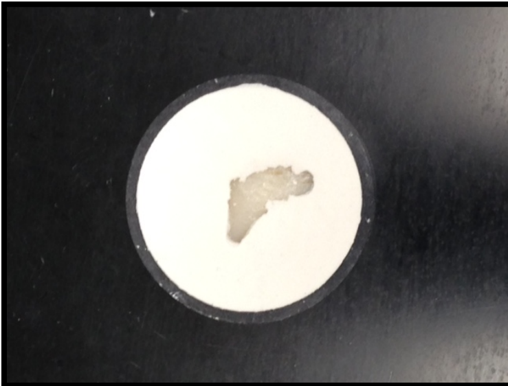
Figure 3-3 Mounted bovine tooth facial surface exposed in ring and white orthodontic stone
