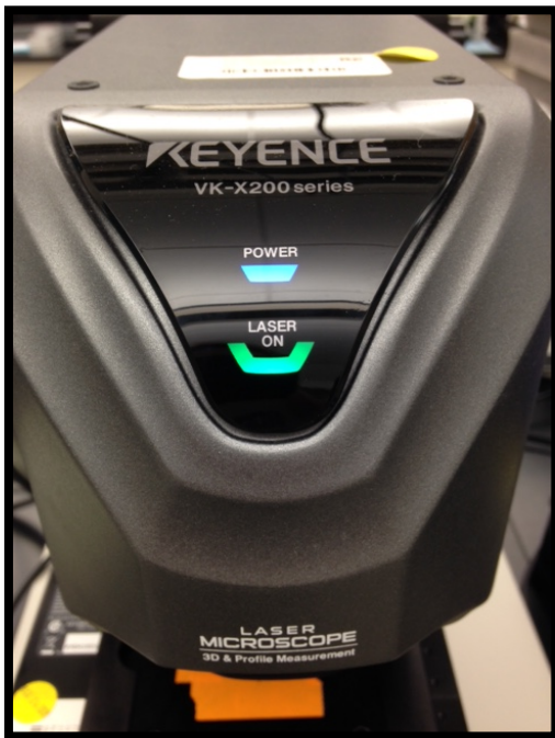
Figure 3-7 Keyence 3D Laser Confocal Scanning microscope used for scanning samples
