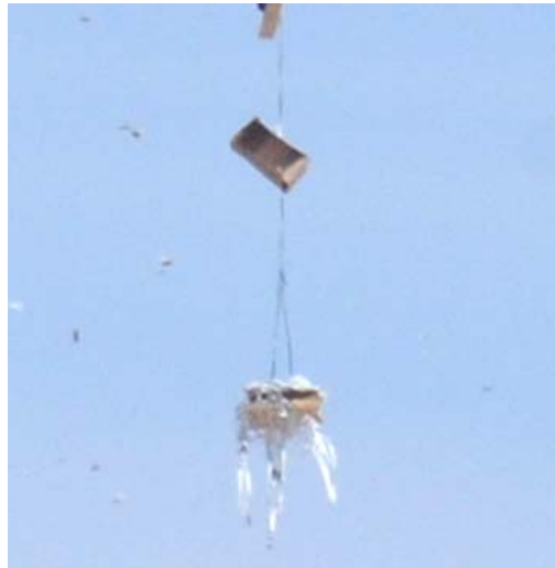
Figure 23: Inverted skid board, foam face down, supported by the supplemental suspension system
