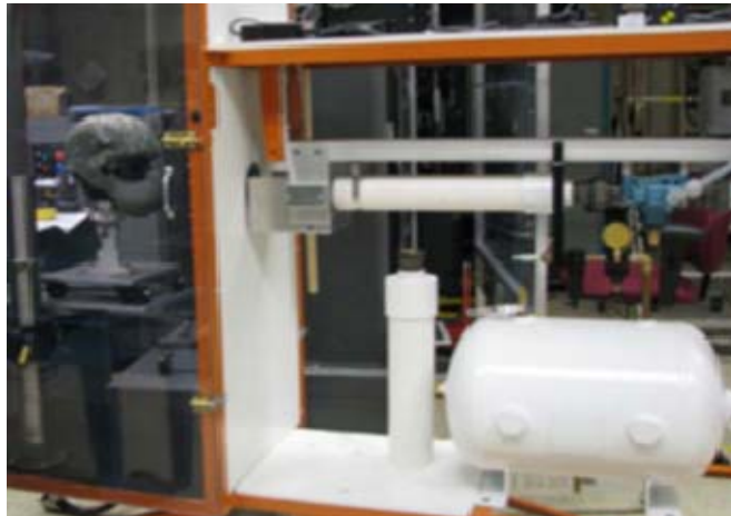
Figure 10: USAARL Accelerated Impact Test Set-up
