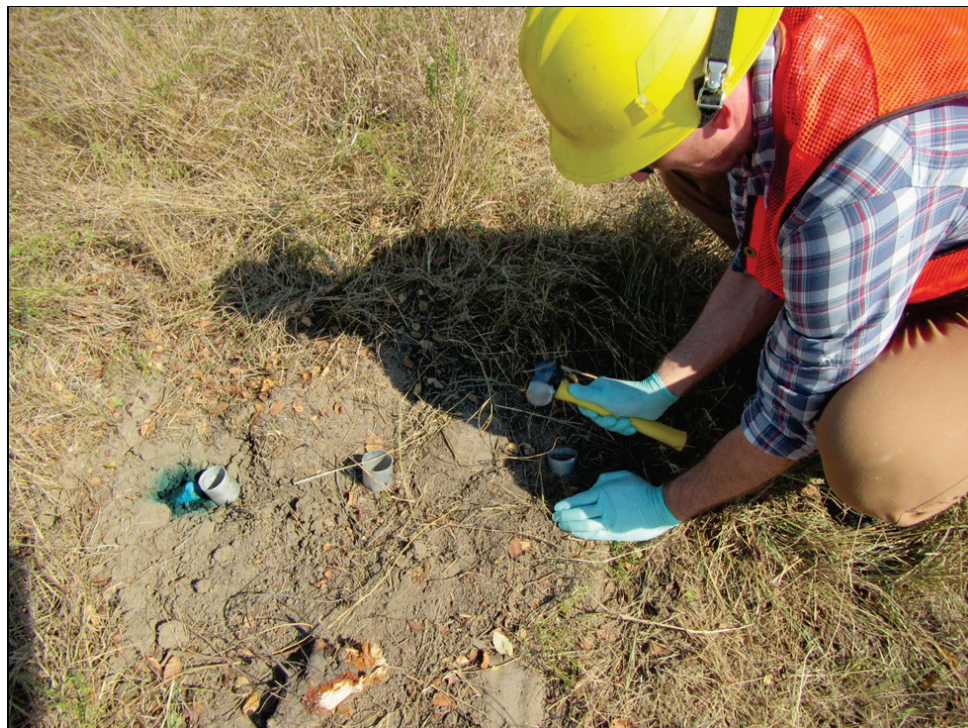
Figure 26. Soil was sampled 61 cm, 30.5 cm, and 0 cm from an herbicide-treated stump.
