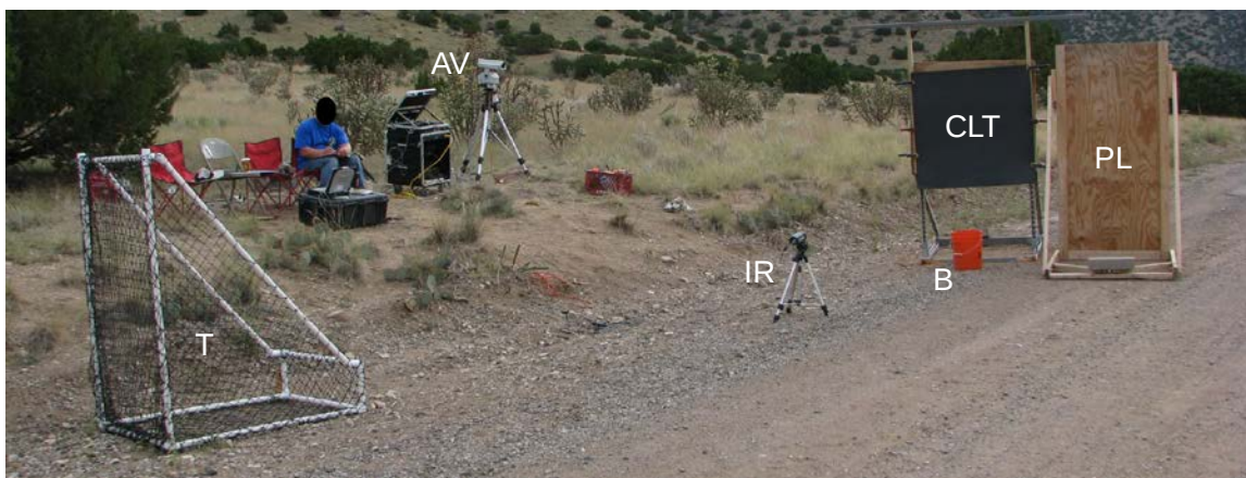
Figure 1. Set-up for Experiment 2. CLT = carbon-loaded Teflon (used for beam characterization), B = bucket of balls, PL = plywood barrier behind which subjects could move, T = target, IR = infrared camera, AV = audiovisual suite used to record subject behavior. During beam characterization, the carbon-loaded Teflon stand is situated where the subject throws balls (as in this figure), but is moved during the subject trials.
