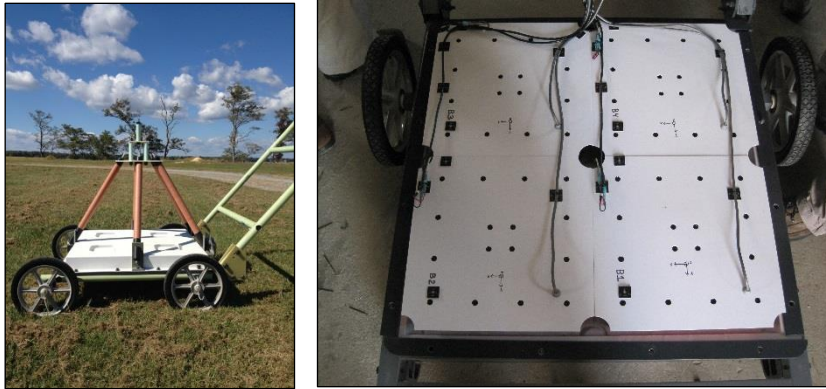
Figure 2. NRL TEMTADS 2x2 (left) cart alone, and (right) with weather shield removed.
