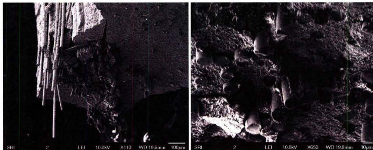
Figure 47. SiC fibers coated with PEDAB embedded in pyrolyzed matrix material.
