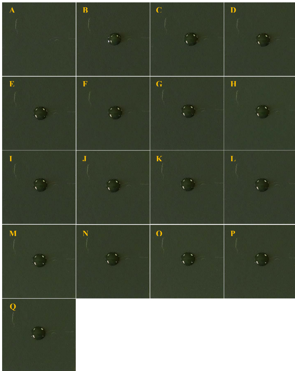
Fig. A3 — DMMP on the C2F6, 50 W, 30 min treatment (1'' x 1'' coupon). Images of a coupon before application (A) and at 0 (B), 0.5 (C), 1 (D), 1.5 (E), 2 (F), 2.5 (G), 3 (H), 3.5 (I), 4 (J), 4.5 (K), 5 (L), 10 (M), 15 (N), 20 (O), 25 (P), and 30 (Q) min following application of the target.
