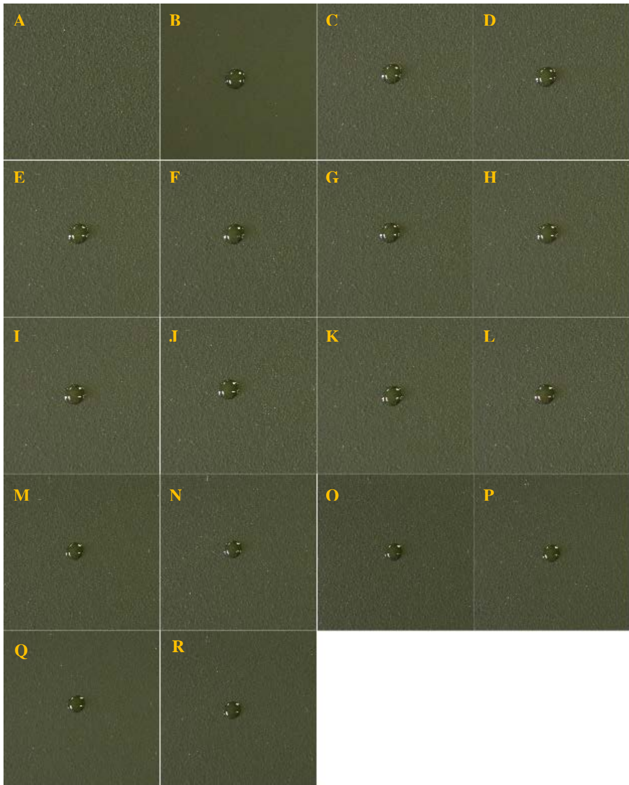
Fig. A6 — DMMP on Nanoskin. Images of a coupon before application (A) and at 0 (B), 0.5 (C), 1 (D), 1.5 (E), 2 (F), 2.5 (G), 3 (H), 3.5 (I), 4 (J), 4.5 (K), 5 (L), 5.5 (M), 10 (N), 15 (O), 20 (P), 25 (Q), and 30 (R) min following application of the target.
