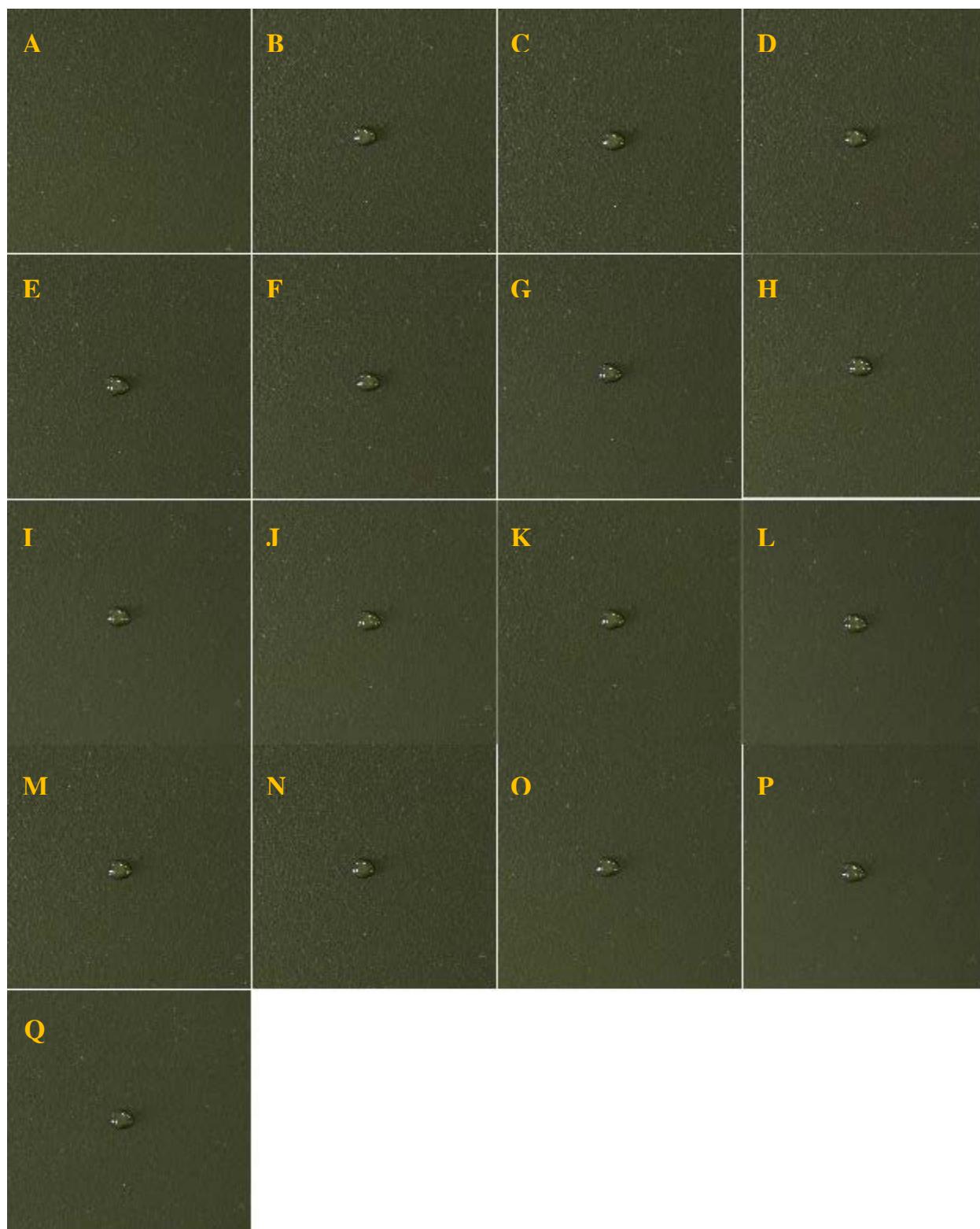
Fig. A5 — MES on Nanoskin. Images of a coupon before application (A) and at 0 (B), 0.5 (C), 1 (D), 1.5 (E), 2 (F), 2.5 (G), 3 (H), 3.5 (I), 4 (J), 4.5 (K), 5 (L), 10 (M), 15 (N), 20 (O), 25 (P), and 30 (Q) min following application of the target.
