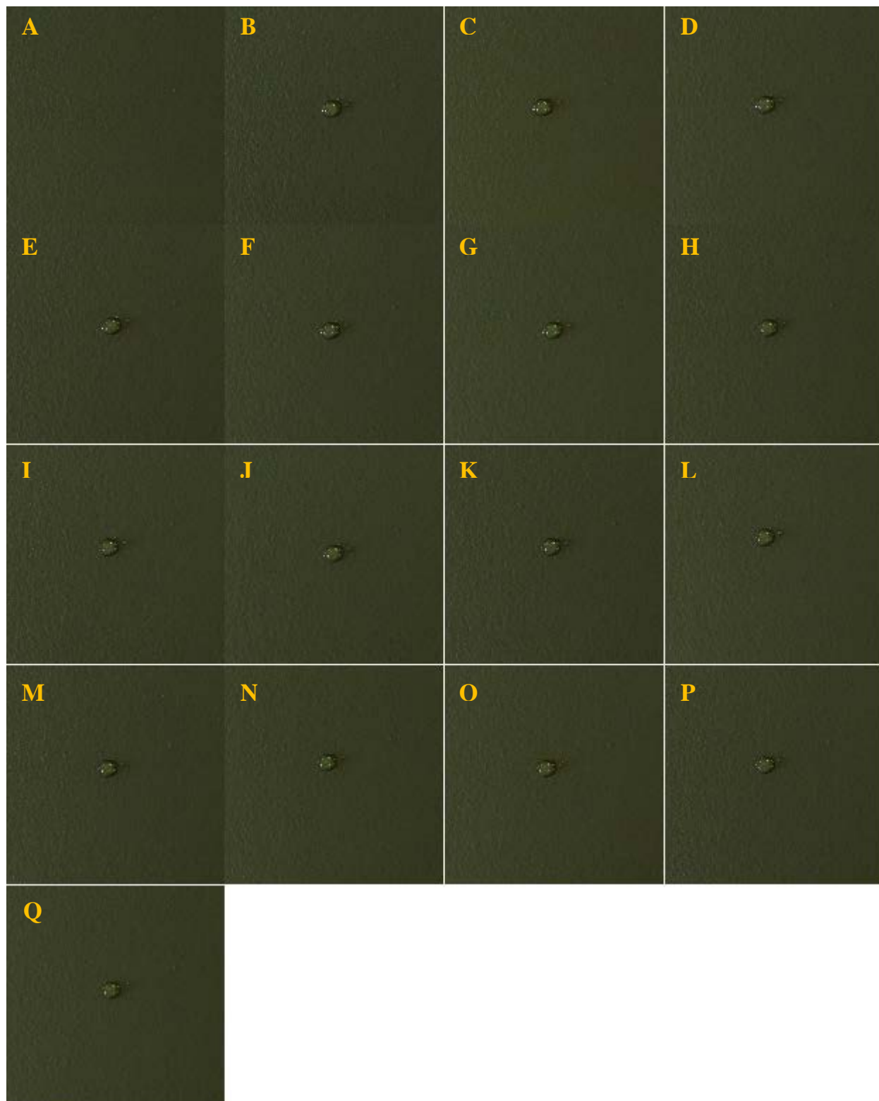
Fig. A9 — DMMP on Wipe New. Images of a coupon before application (A) and at 0 (B), 0.5 (C), 1 (D), 1.5 (E), 2 (F), 2.5 (G), 3 (H), 3.5 (I), 4 (J), 4.5 (K), 5 (L), 10 (M), 15 (N), 20 (O), 25 (P), and 30 (Q) min following application of the target.
