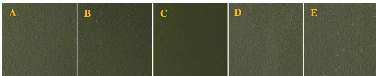
Fig. 1 — Images of a painted coupon (A), a Nanoskin treated coupon (B), a Wipe New treated coupon (C), a NeverWet treated coupon (D), and a NanoWax treated coupon (E).
