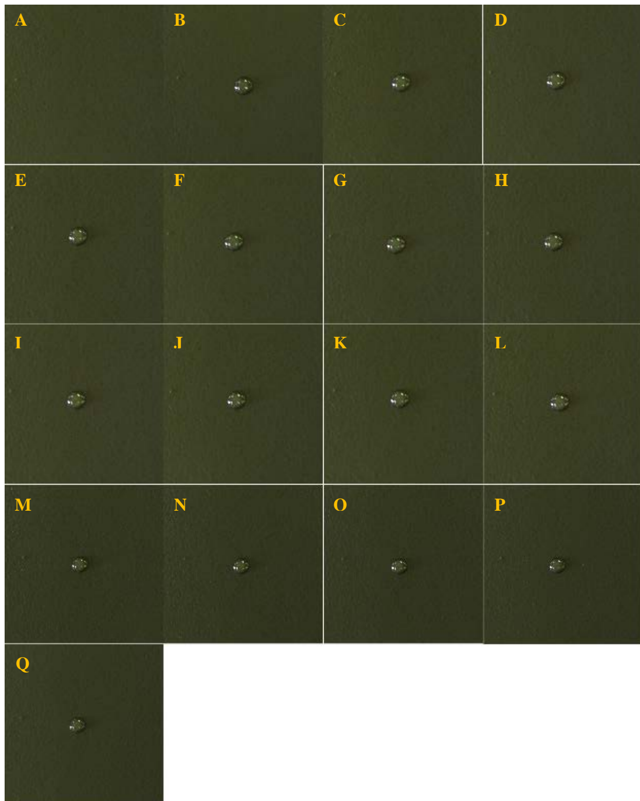
Fig. A8 — MES on Wipe New. Images of a coupon before application (A) and at 0 (B), 0.5 (C), 1 (D), 1.5 (E), 2 (F), 2.5 (G), 3 (H), 3.5 (I), 4 (J), 4.5 (K), 5 (L), 10 (M), 15 (N), 20 (O), 25 (P), and 30 (Q) min following application of the target.
