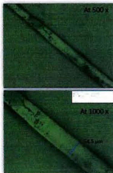
Figure 23: Digital optical microscope images of small-size square cross-section Nafion fibers fabricated using slicing method.
