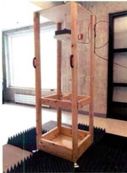
Figure 1.1. Wooden frame holding reader, antenna, and RFID tags above a floor of electromagnetic absorbers.
