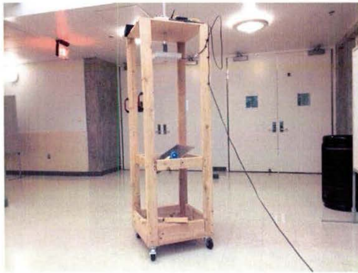
Figure 2.10. Experiment setting for the measurement of RSSI versus angle relationship.
