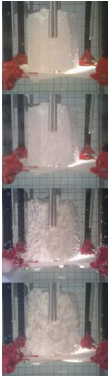
Figure 28. TNGU-LMA PBX test item while being submerged in water for 1 min, 1 h, 12 h, and 24 h.
