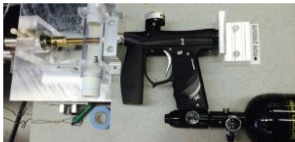
Fig. 6. A miniature cannon for blast-induced trauma to the eye. The apparatus consists of a paintball gun (1) (without paintballs) with a customized barrel (2), a tube to hold the mouse (3), and a Honeywell pressure transducer to calibrate the force of the pressure wave (4).
