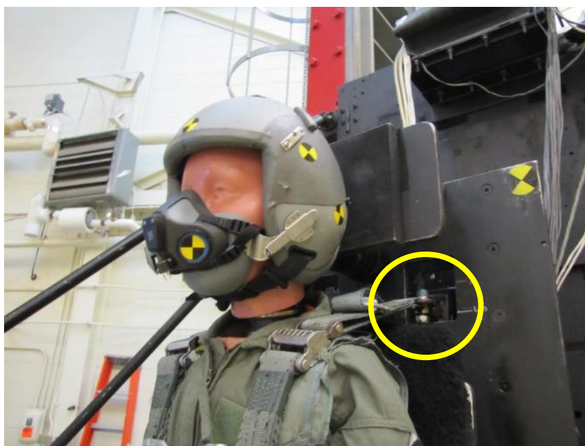
Figure 5. Location of Shoulder Belt Tri-axial Load Cell on Generic Seat Fixture
