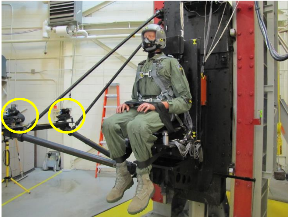
Figure 8. Phantom Miro-3 Cameras Mounted On-Board VDT Carriage
