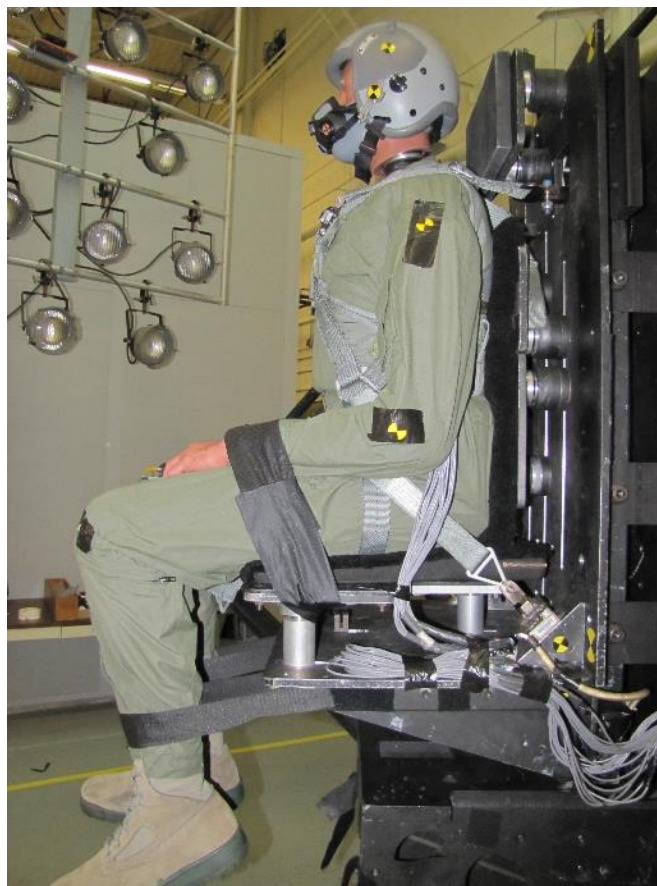
Figure 2. Generic Seat Fixture Mounted to Front of VDT Carriage
