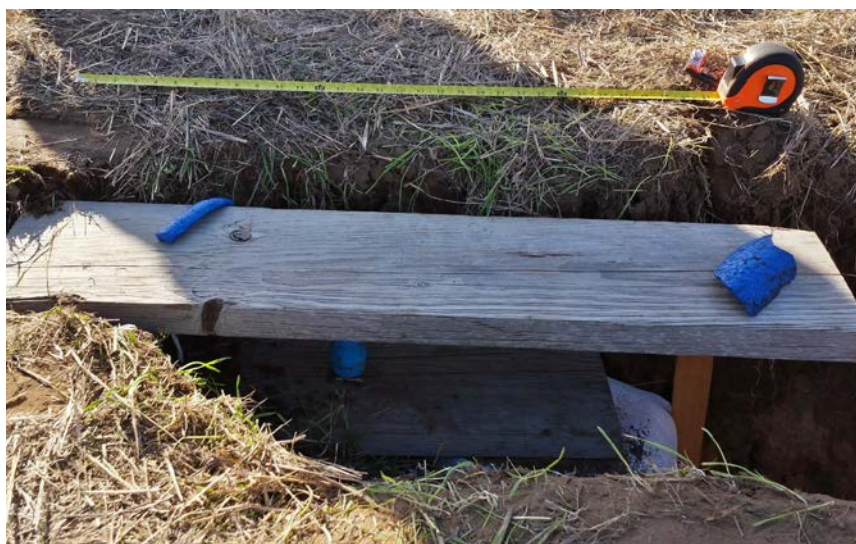
Figure 5-3: Example of a Test Pit Measurement of a 40mm Projectile at 8 inches Depth and Frag Near to the Surface
