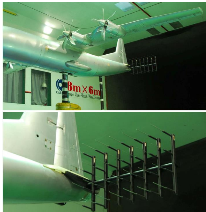
Figure.2 Flow field test with seven-hole probe rake
