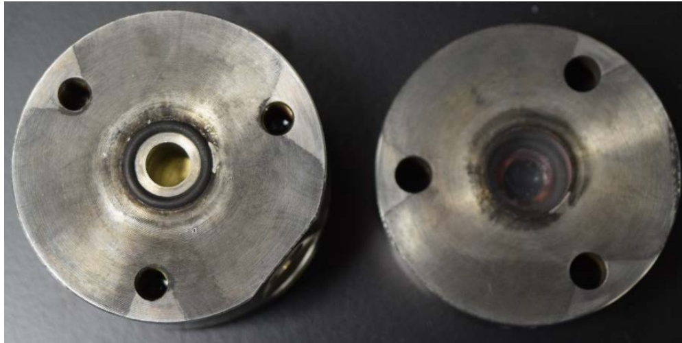
Fig. 5 Extreme example of blow-by at the window seal. The chamber was filled with 50 mg of JA2 scrap and leaked due to seal failure at a pressure of about 40 MPa.
