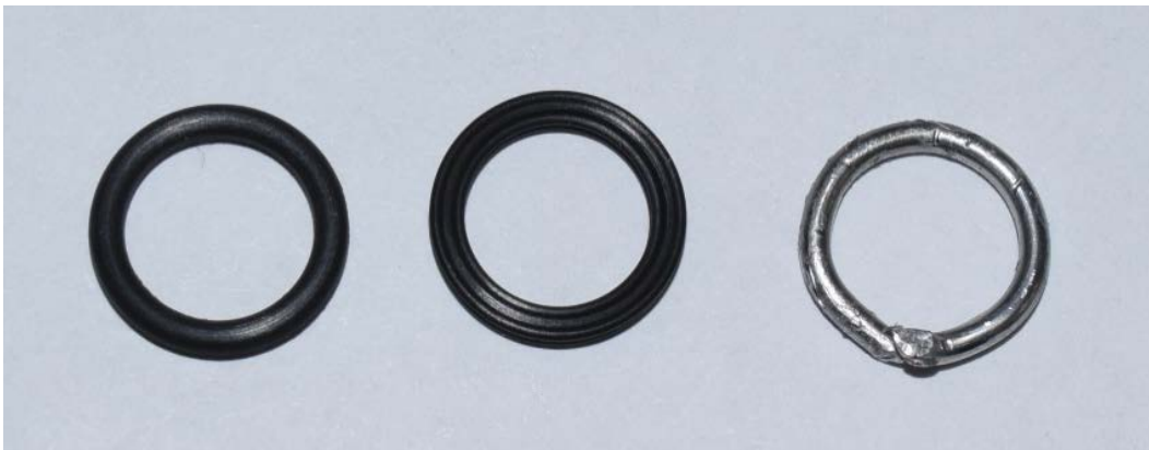
Fig. 9 Conventional O-ring (left), X-section O-ring (center), and solder ring (right). The O-rings, sized -012, have an outer diameter of 12.7 mm and an inner diameter of 9.5 mm.
