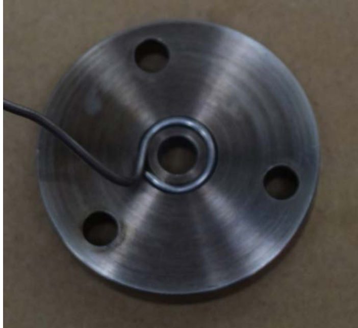
Fig. 8 Fabrication of a solder window seat using an O-ring groove in the diaphragm flange
