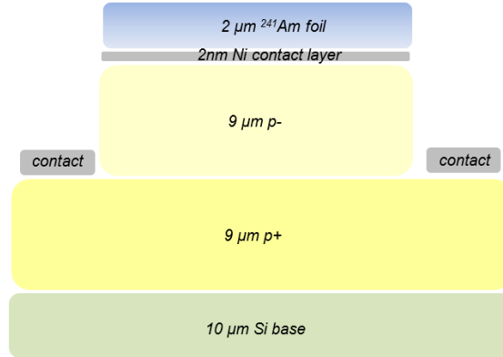
Fig. 8 Quasi-vertical diamond device designed to match energy deposition
