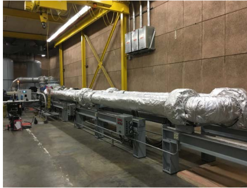
Figure 5-1 AFRL Mach-6 Ludwieg Tube Hypersonic Wind Tunnel.
