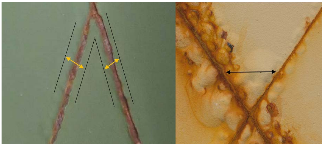
Fig. 2 Creep originating from each side of the scribe (left) and of indeterminate origin (right)
