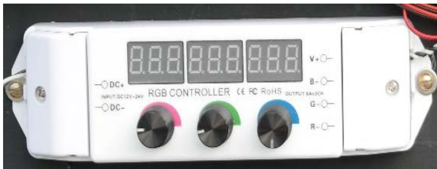
Fig. 6 LDKR-RGB6 PWMs with 3 pulse-width modulation circuits
