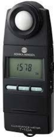
Fig. 2 Konica Minolta T-10A illuminance meter. Used with permission from Kyle Drozenski (Kyle.Drozenski@konicaminolta.com).
