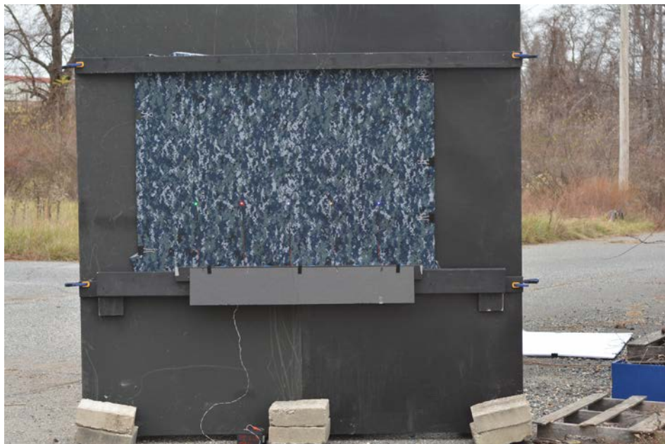
Fig. 10 Outdoor testing display shown with the MARPAT Navy camouflage pattern and illuminated LEDs
