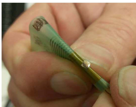
Fig. 3: Substrate Failure at 2.5mm RoC
