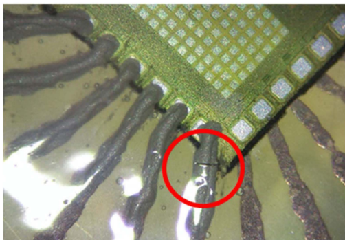
Fig. 7: Crack in Printed Interconnects on VDD Line
