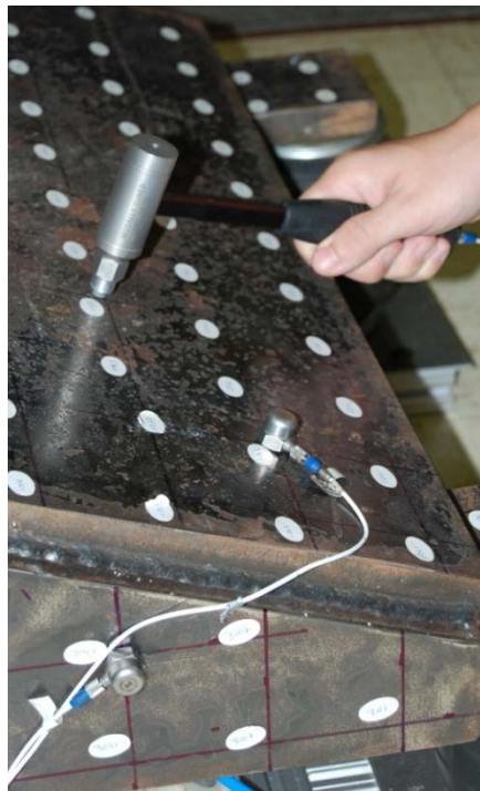
Fig. 5 Roving hammer test
