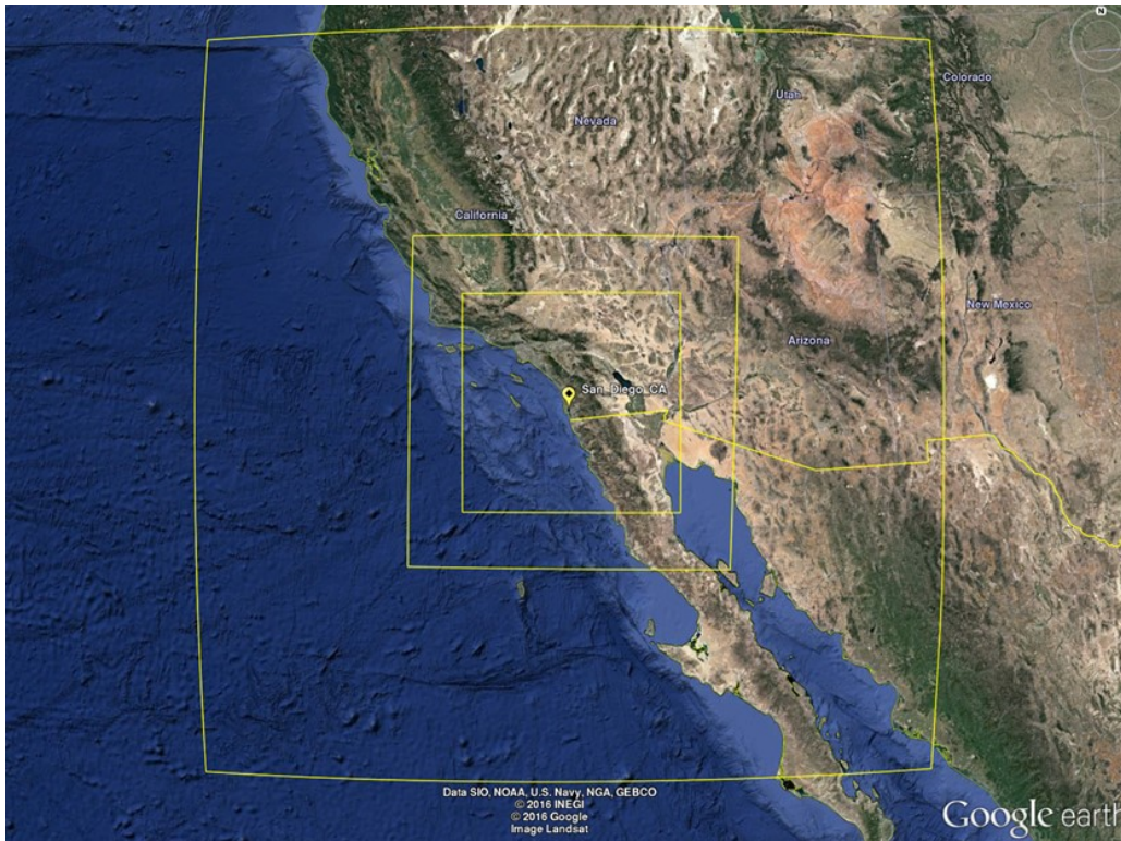
Fig. 1 Triple-nested model domains: domain center points are coincident and are centered near San Diego, CA (Google Earth 2016)
