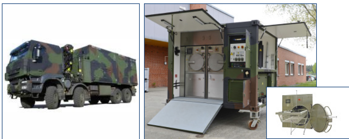
Figure 3-13: Sensitive Equipment Decontamination System (WIS).
