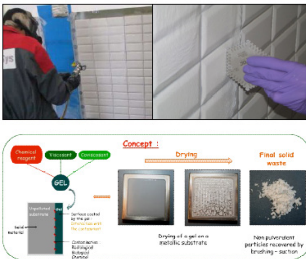
Figure 3-18: Example of Vacuumable Gels (F. Cuer and S. Faure, http://www.agence-nationale-recherche.fr/Colloques/WISG2013/presentations/AAP10_GIFT-RBC.pdf ).
