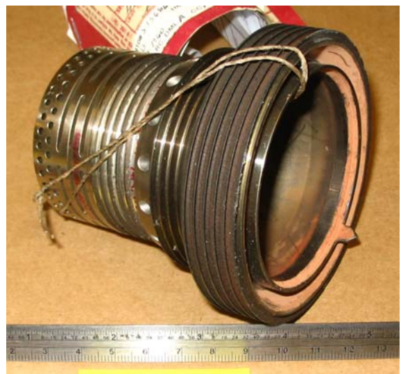
Figure 5.—Modified compressor discharge pressure seal with impacted sand.
