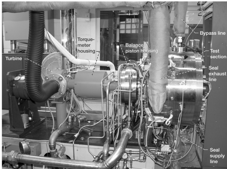
Figure 12.—NASA High Temperature, High Speed Turbine Seal Test Rig.
