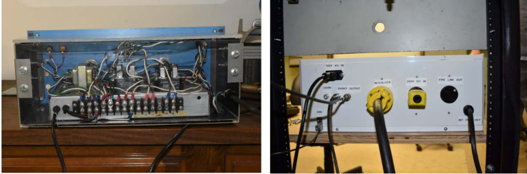
Fig. 2 Rear-face view, old (left) and new (right) fire switch and relay box. Note the reduced wiring on the new fire switch and relay box, elimination of finger protection, and elimination of the electric bus bar.
