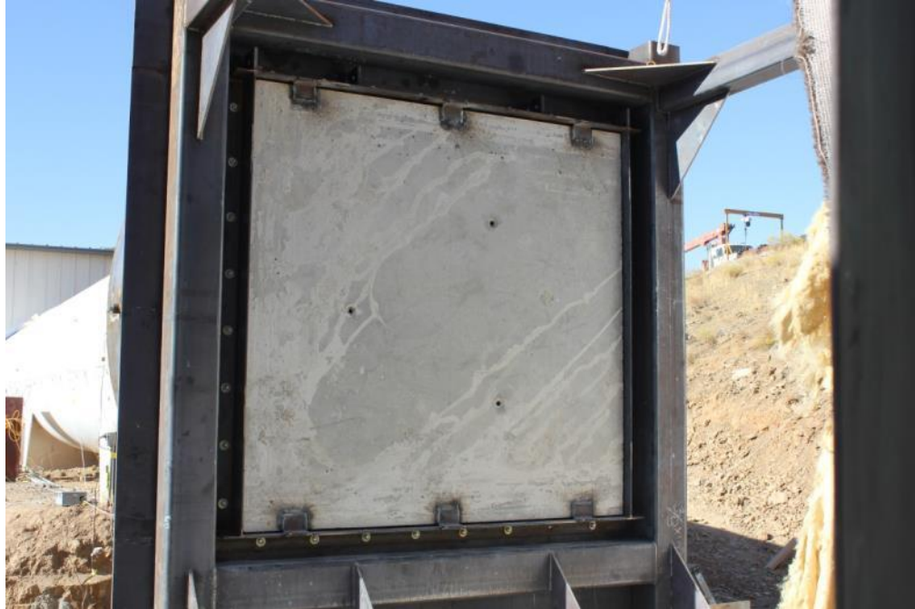
Figure 6. A view of concrete panel sample set-up used in Test 21.
