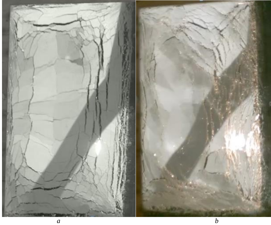
Figure 12. Glass fragmentation approximately 10ms after the airblast arrived for a) Test 17 and b) Test 19.
