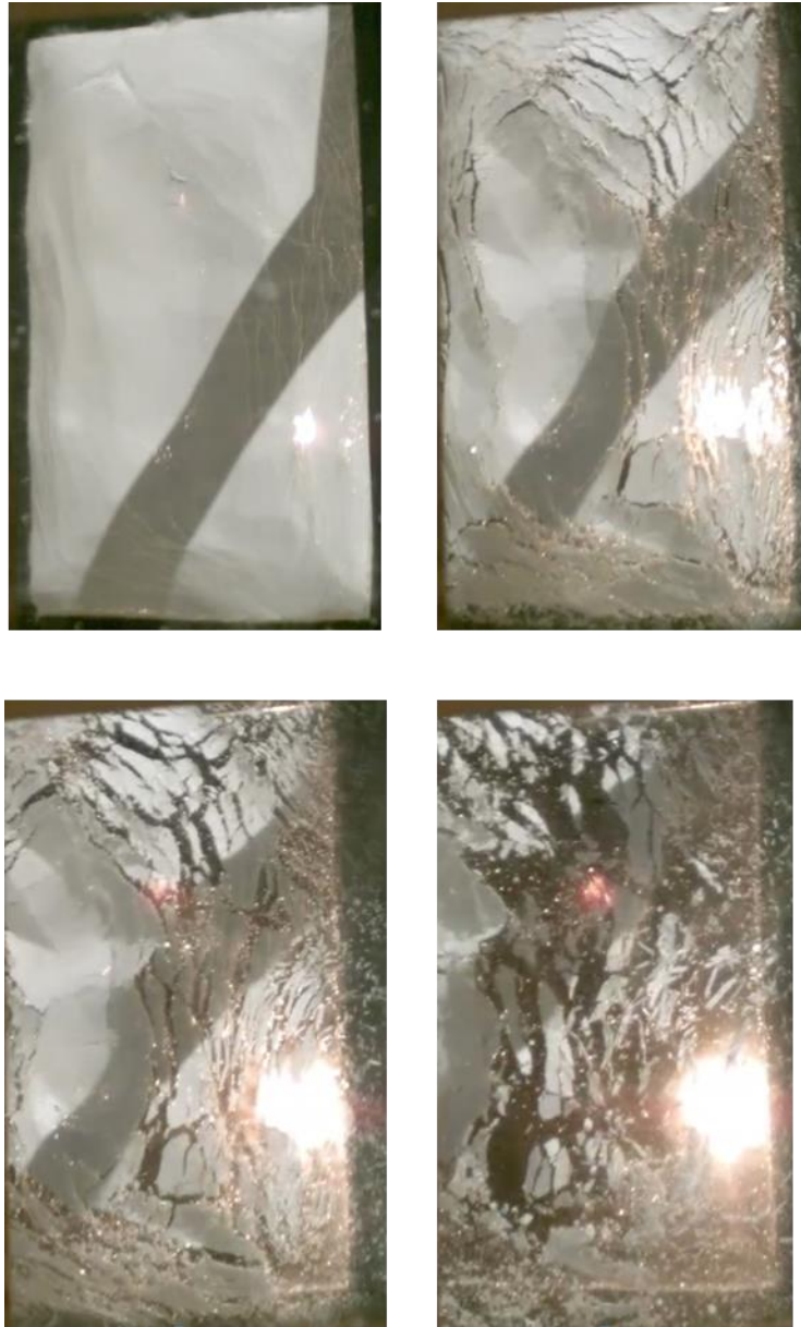
Figure 14. Glass fragmentation in Test 19 at 0ms, 5ms, 10ms, and 15ms after the shock arrived.
