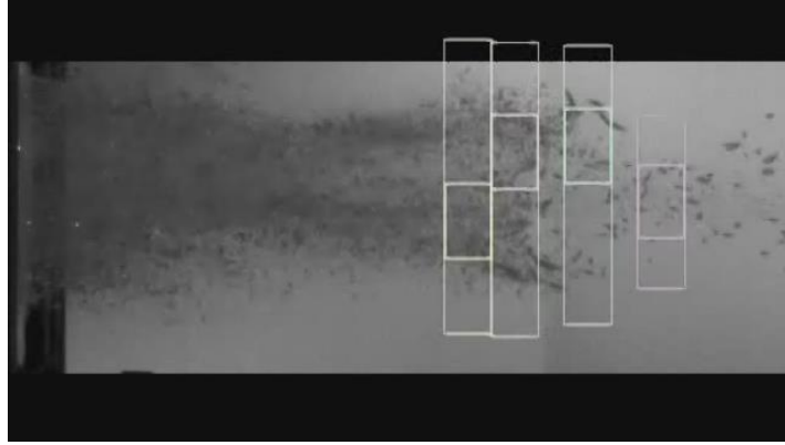
Figure 21. Frag Track used to estimate airborne fragment velocities from side-view HSV.
