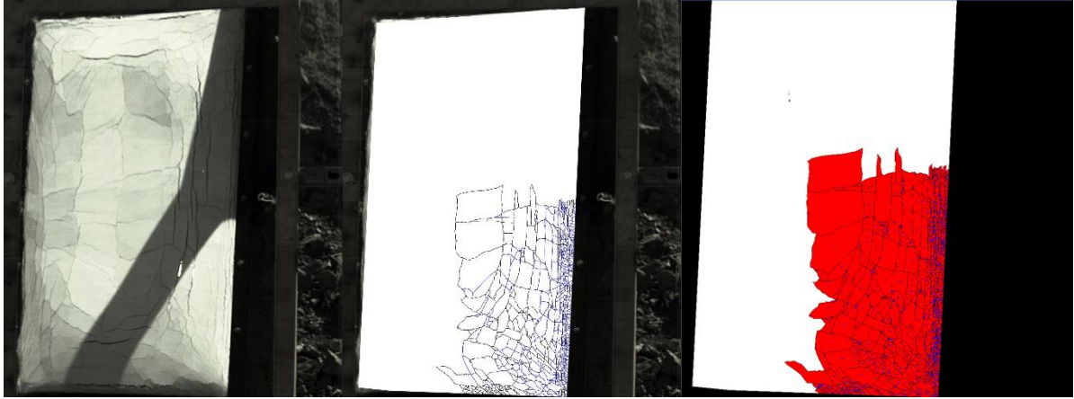
Figure 19. Progression of image analysis for size distribution using SigmaScan for Test 17.
