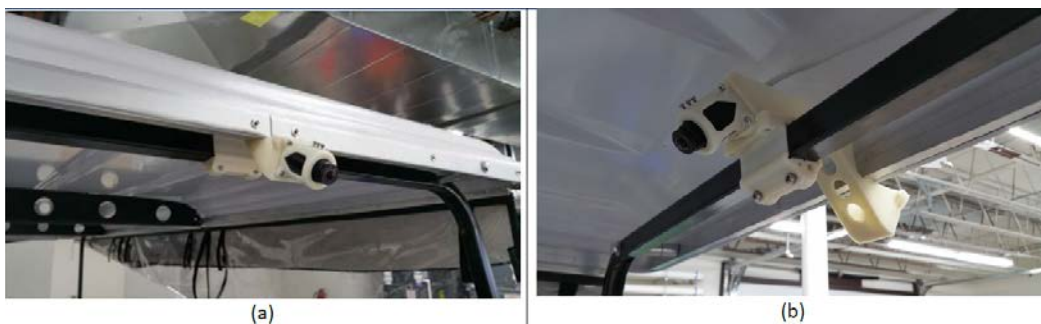
Fig. 5 a) Forward-facing and b) passenger-facing cameras
