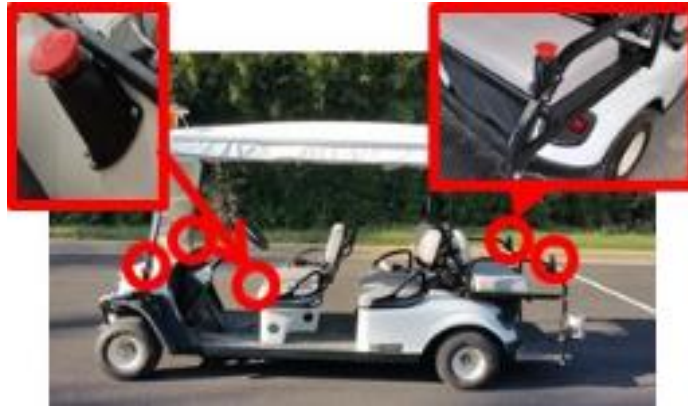
Fig. 6 Placement of e-stop buttons
