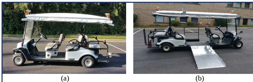
Fig. 3 ARIBO driverless vehicle variants: a) 6-passenger and b) Americans with Disabilities Act (ADA)-compliant wheelchair accessible models
