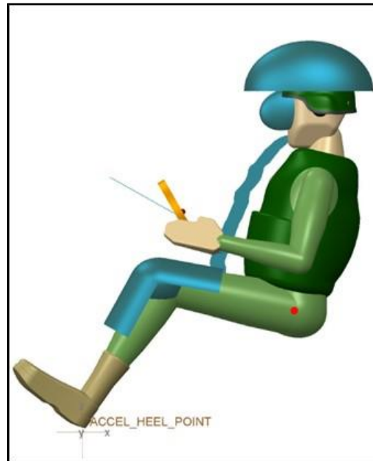
Figure 10: Manikin Placement Using Posture Prediction Model
