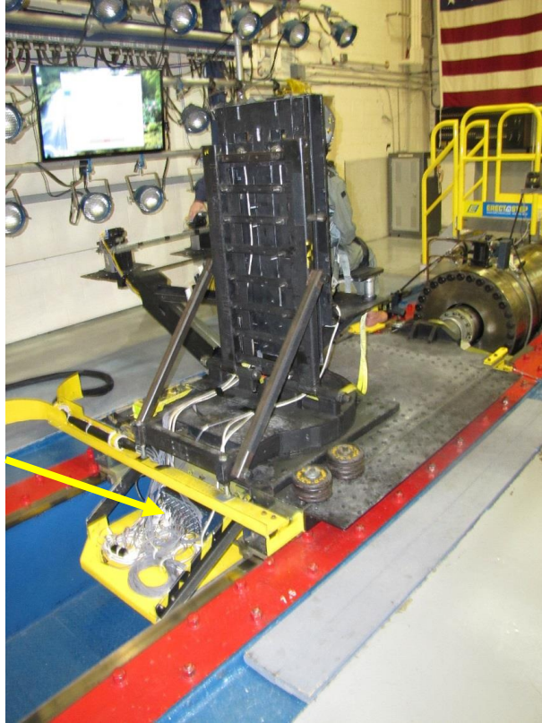
Figure 8. Location of TDAS PRO Data Collection System Mounted on HIA Sled
