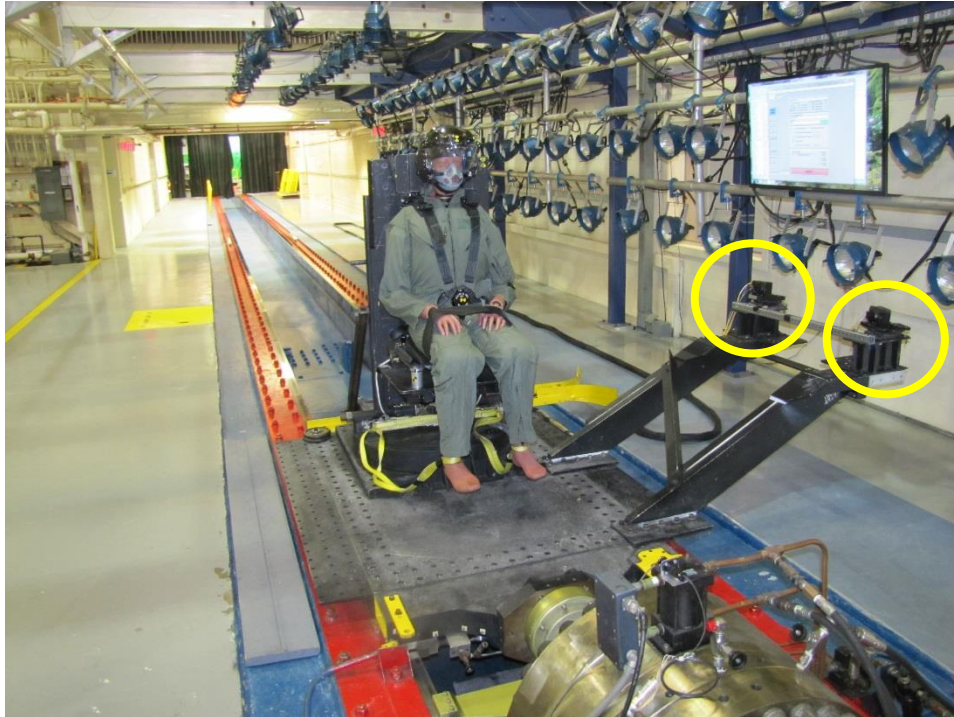
Figure 10. Phantom Miro-3 Cameras Mounted On-Board HIA Sled
