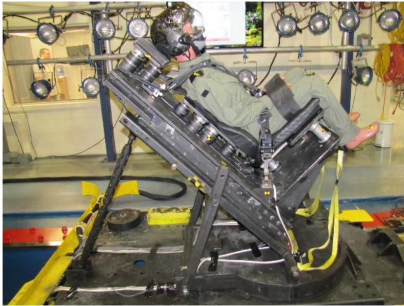
Figure 3. Generic Seat Fixture Mounted in Reclined Position on HIA Sled
