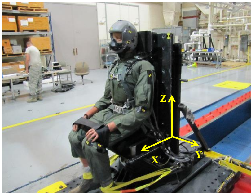
Figure 4. Coordinate System Used for Generic Seat Fixture on HIA Sled
