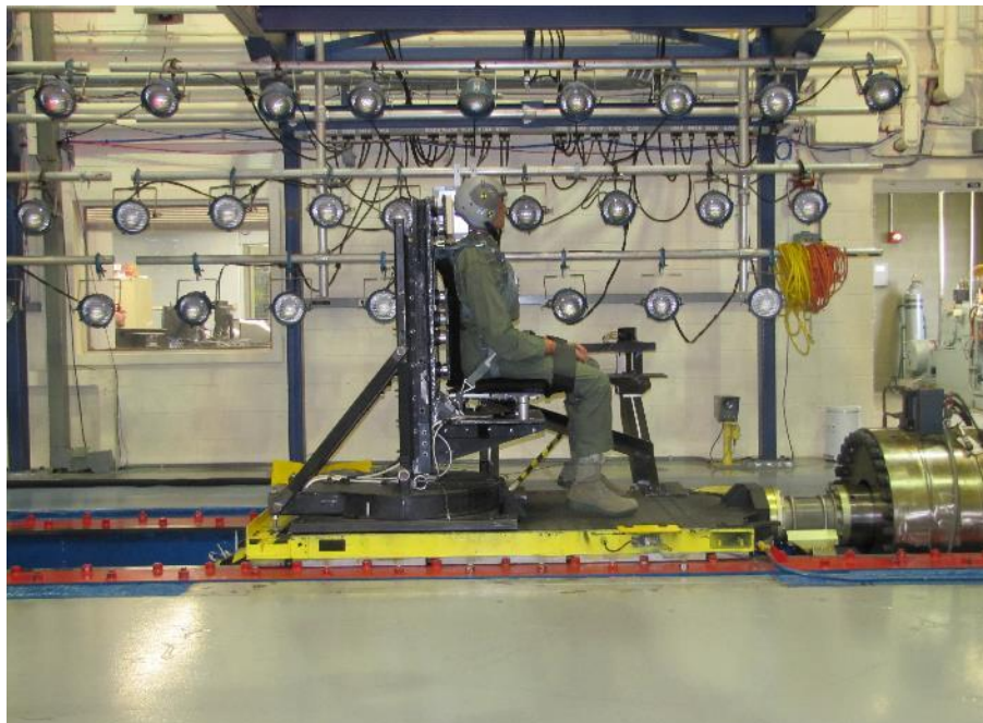
Figure 2. Generic Seat Fixture Mounted in Upright Position on HIA Sled
